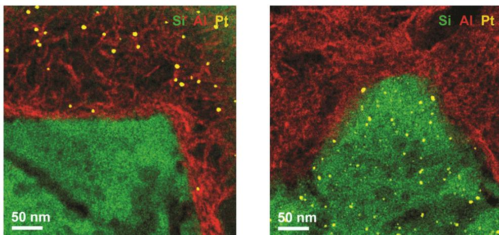
In our most recent research (with zeolite ZSM-5), the Pt/Al<sub>2</sub>O<sub>3</sub>/zeolite catalyst is more active when the Pt nanoparticles are present on the alumina binder than when the Pt nanoparticles are present in the zeolite. Provide a working hypothesis why this is. Also propose an experiment to (dis)prove your working hypothesis. **[20 points]**
